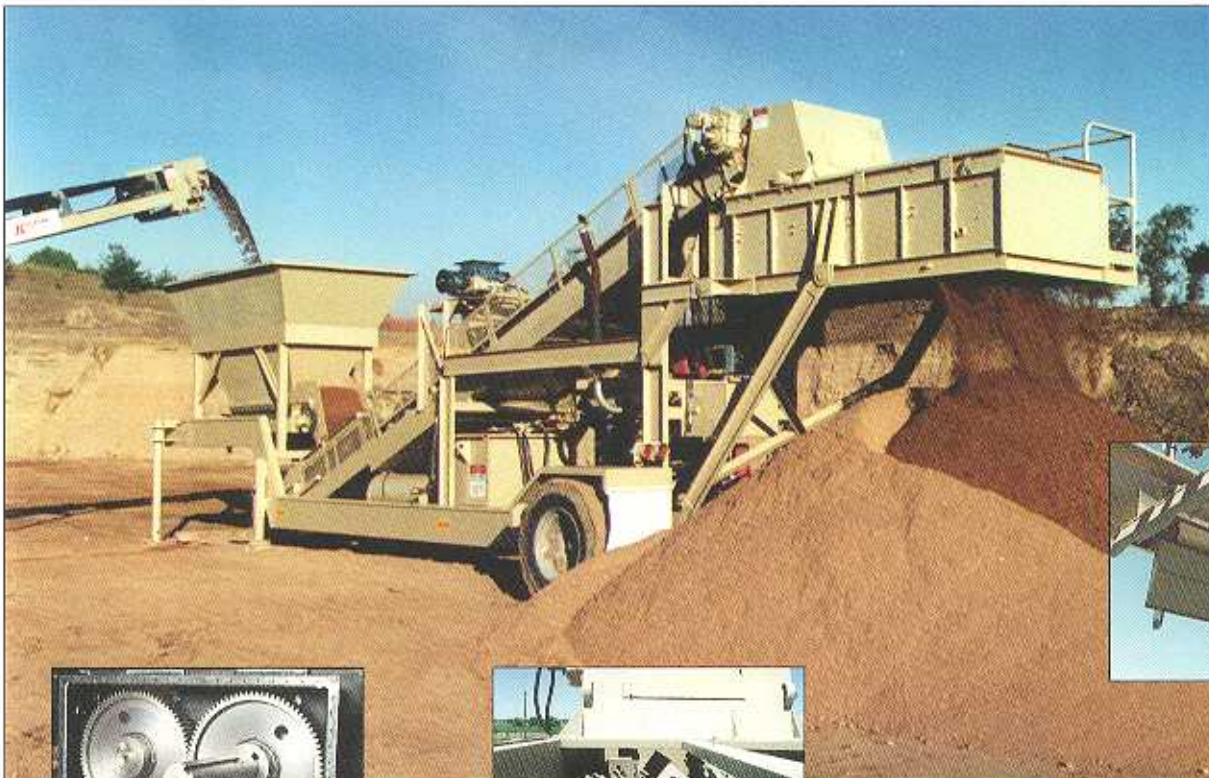
ADJUSTABLE/REVERSIBLE PADDLES: All Pugmill paddles are standard Ni-Hard wear resistant steel. The paddles are adjustable to six (6) positions on the arms to increase retention time and improve mixtures as well as increasing wear life.
